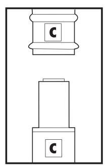
4. INSERT LAMP INTO POLE, MATCHING "C" TO "C". TWIST TO LOCK.
